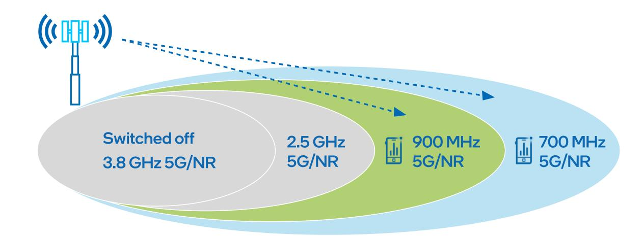
**Figure 2:** In times of high traffic (top image), all carriers are on. High-band carriers are switched off when traffic is low, and users are moved to low-band carriers.
