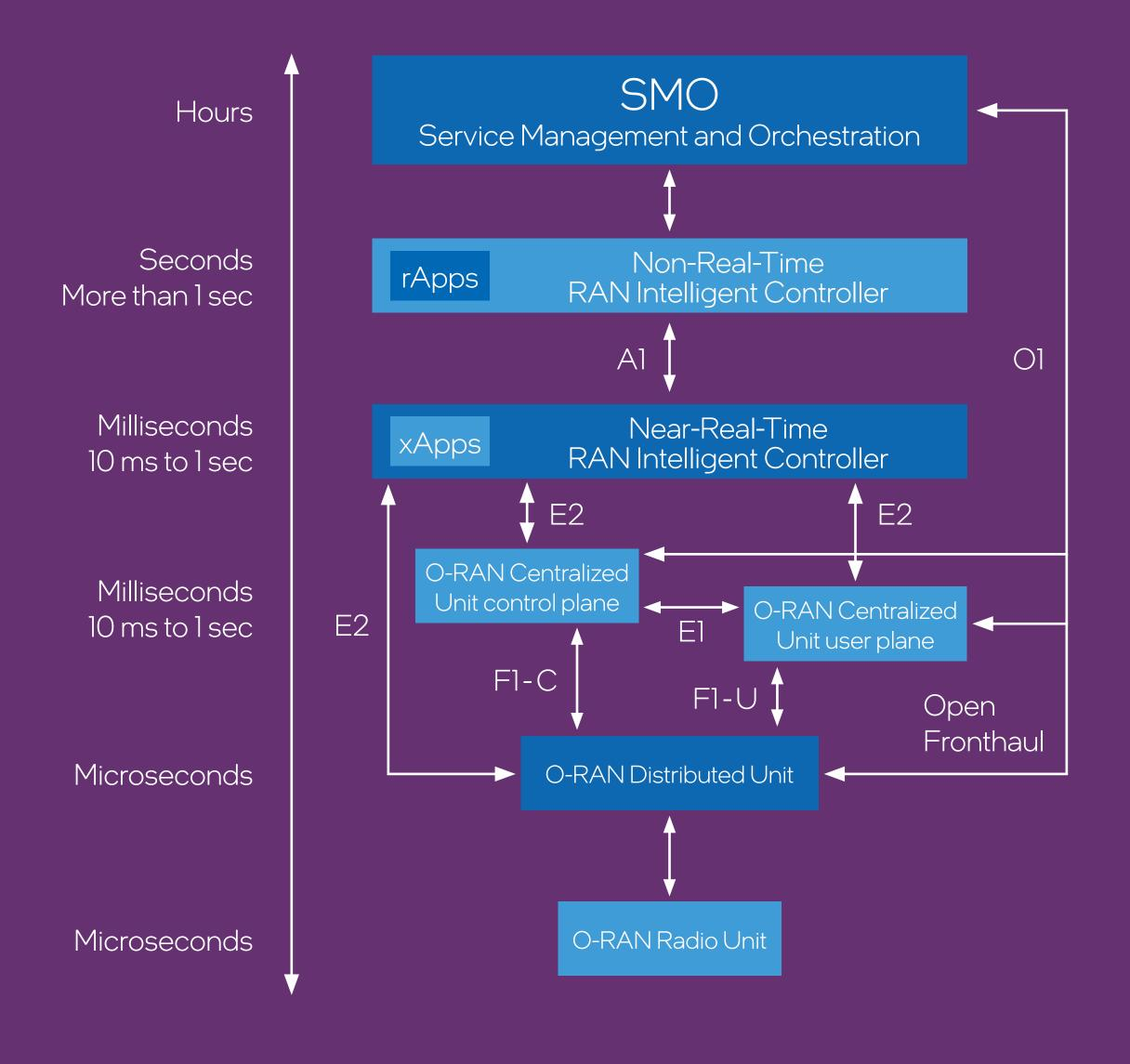
**Figure 1:** The O-RAN Intelligent RAN Architecture, showing the different functions, the latency for each one, and standardized interfaces between them for data collection and policy communication.
